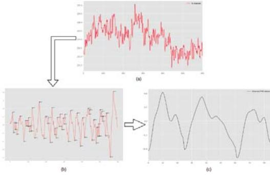
Fig. 3. (a) Time series of the red channel, (b) PPG waves, (c) Selected best three PPG waves. For feature extraction, we generated Photoplethysmography (PPG) for each subject's fingertip video.
