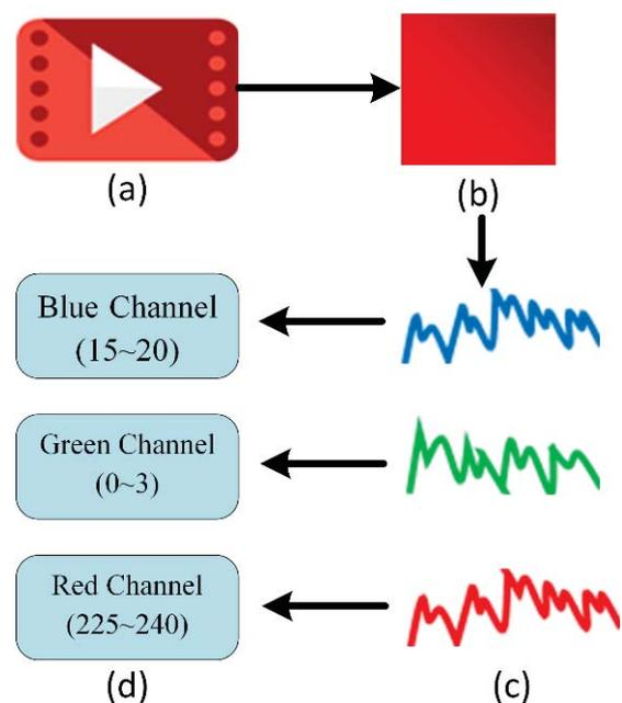
Fig. 2. (a) Raw video that was taken with Google pixel-2 smart-phone. (b) Extract frames: Cropped frame (500x500) pixel from right to left section of extracted frame (1920x1080) pixel. (c) Time series plot of average intensity for 3 channels from all cropped frames. (d) Intensity range classification.
