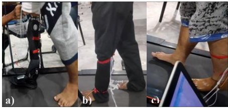
Fig 8 : Hardware implementation and 3-way data collection: a) With Prosthetic Exo-leg, b) Healthy human walking, & c) With poly acrylic leg
