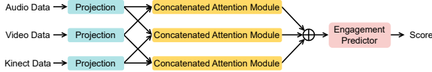
Fig. 2. An overview of the proposed TCA-Net model: the embeddings of three modalities are standardised in scale and proceeded modality-specific learning through projectors. The computed modalities are fused pairwise using the proposed concatenated-attention modules. The fused results, once concatenated, are then passed into the predictor for prediction.
